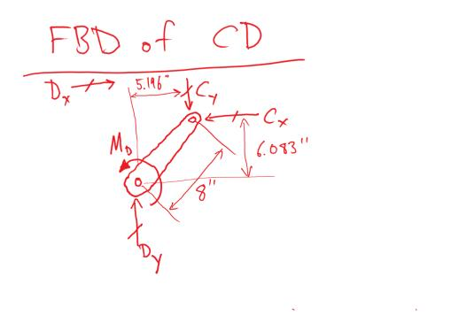
$$(\Sigma M)_{D} = 0 = M_{D} - (5.196'')C_{Y} + (6.083'')C_{X} = 0$$
